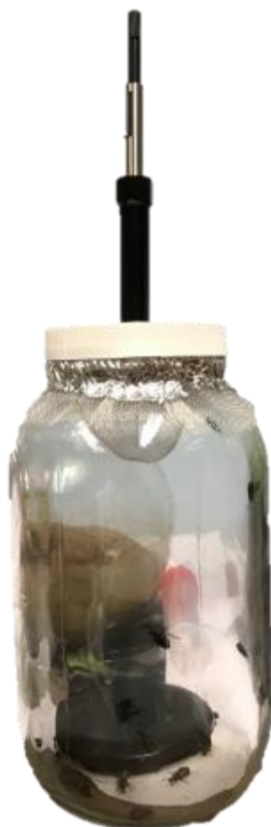
Figure 11. A two litre glass sample container sealed with a PTFE-lined screw cap lid retrospectively fitted with a PTFE septa with SPME fibre inserted into container.
